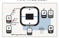
Note: This feature can be used with any combination of FAN Speeds, Timer, or Sleep Modes. When in the "Heat" Mode, the fan will run continuously while heat is needed. The temperature will automatically be maintained anywhere between 55°F (13°C) and 80°F (27°C). When the room set temperature is satisfied, the fan will cycle off and on to circulate and sample the room air.
